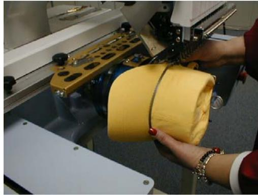
15. Move current needle (red dot needle), with the jog keys to center of cap.
