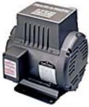
The third choice is to use a Rotary Phase Converter. These look like motors, because, they are! They have a motor and additional windings that generate the other 2 phases needed by the machine.
