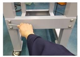
9) Tighten the button bolts on all (3) Joint Brackets.
