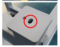
6) Install the CBIII on the top of the cart. Insert the (4) hex socket bolt heads on the bottom of the CBIII, into the (4) elongated holes on the top of the cart (See photos to the left).
