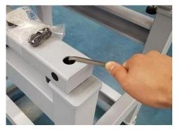
8) Please tighten the (4) M10x30 bolts that were inserted in the previous step 7.
