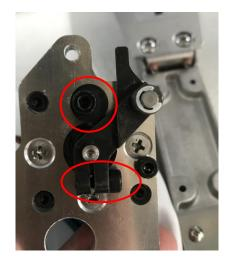
(6) Position the jump lever so it's parallel with the bracket as shown in the photo below. Also set the gap between the bracket and the jump lever to 0.5mm. Tighten the jump lever to hold this position.
