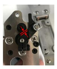
(6) Press the Jump Icon a few times on the screen to see if the lever moves smoothly. When removing or replacing the jump lever, make sure to insert the end of the spring into the split part of the jump lever.
