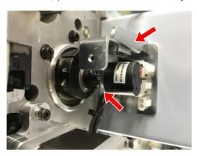
(1) Release the 3 white locking tabs as shown in the photo gently with a small screwdriver and pull the encoder away from its base.
