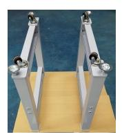
② Attach the front and back joint brackets temporarily to the base stands. Leave the bolts loose at this moment. Later they will be tightened.
