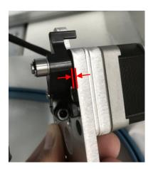
(7) Adjust the stopper so there is a 0.5mm gap between the jump lever and stopper as shown below. Tighten the stopper in place.
