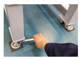
When not using the stand, please level the machine using the adjuster in the following photo.
