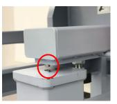
⑤ Attach the CBⅢ to the stand with the M10x30 Hex socket bolts in the accessories. Use the following tightening order shown below.
