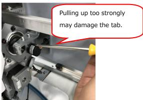
(2) Pull the cable out the machine frame, and unplug the connector to replace the encoder.
