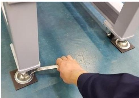
When not using the stand, please level the machine using the adjuster in the following photo.
