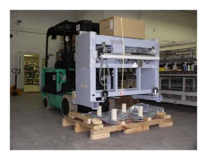
8. While the machine is in the air, remove the wheels and place them in the correct position. As well place the leveling bolts (located on the bottom left support beam in bubble wrap) through the threaded holes in the feet. Ensure that they are in the full up position allowing the machine to roll freely.
