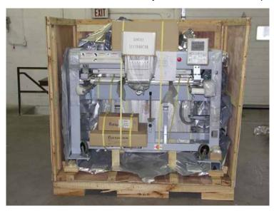
4. Using a pry bar or a hammer, remove the nails to allow for the removal of the back and side panels from the crate.
