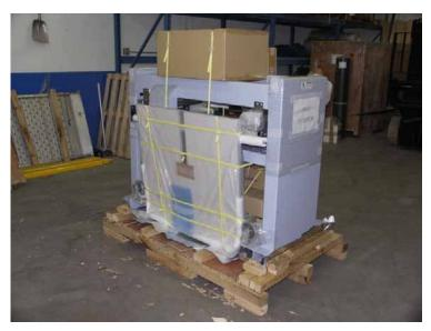
6. Remove the 4 bolts on the feet that are holding the machine to the skid, using a 20mm wrench.
