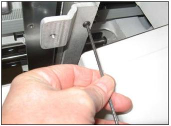
Install **adapter bracket** using 2-M5x12 Button head screws and tighten. (bracket will remain on machine)
