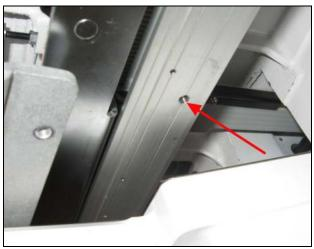
Looking under pantograph, locate 2- M5 tapped holes. (one on each side of cylinder bed)
