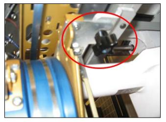
Make sure slotted tabs are seated against knob bolts circled. Tighten, then check pantograph movement front to rear.
