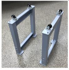
2. Attach the front and back Joint Brackets temporarily on base stands. Do not tighten at this point. Use the "M12x20 Hex socket button bolts" and "M12 Plain Washers" to attach.
