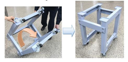
5. Mount the Power unit base to the cart temporarily with "M12x20Hex socket button bolts and washers".
