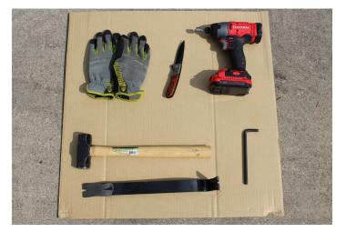
2. The tools needed to uncrate the machine: drill with 10mm socket, hammer, pry bar, knife and gloves.
