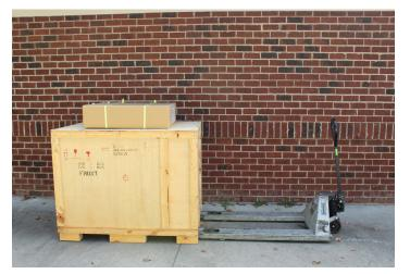
3. The machine cart is boxed and banded to the top of the crate. Cut the bands and place the box on the ground. Open the box and unwrap the five pieces for assembly.
