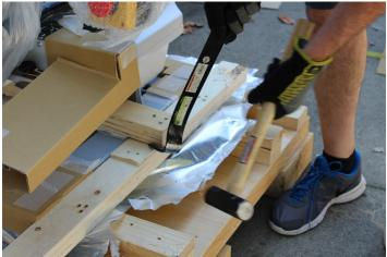
10. With the hammer and pry bar, carefully remove all of the wooden hold down supports from all sides of the machine. Once the hold down supports are removed, the machine will be free from the pallet and ready to be carefully positioned on the cart. Please use assistance when moving the machine.
