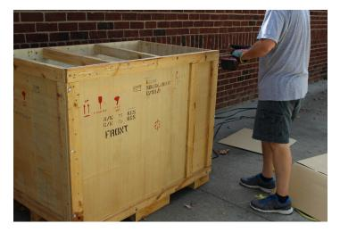
7. Once the top of the crate is off, remove the cap accessories and set them aside. Remove the lag screws holding the two wooden beams that supported the top of the crate. The beams are nailed from the back of the crate, so just pry them up and push them to the rear, out of the way. Remove the lag screws from the front of the crate and discard the front panel.
