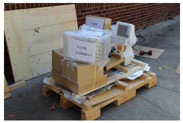
9. With the sides of the crate removed, cut the yellow banding and set the accessory boxes and thread stand (packed in bubble wrap) aside.
