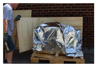
8. The remaining sides of the crate are nailed. Using the hammer and pry bar, remove the three sides and discard. Next, carefully cut the moisture barrier as close to the bottom of the machine as possible. Remove and discard the moisture barrier.
