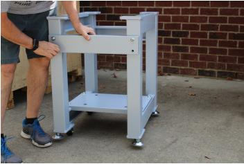
5. Assemble the cart with the provided bolts and washers. Use an 8mm hex wrench to tighten the bolts. It should look like this when it is assembled.
