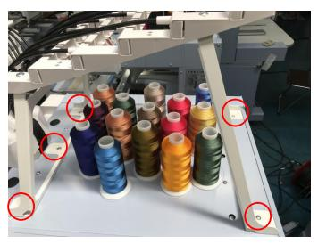
② Mount the thread guide base assembly to the tension base and attach with (4) M3x8 cap bolts in the following red circled areas shown below.
